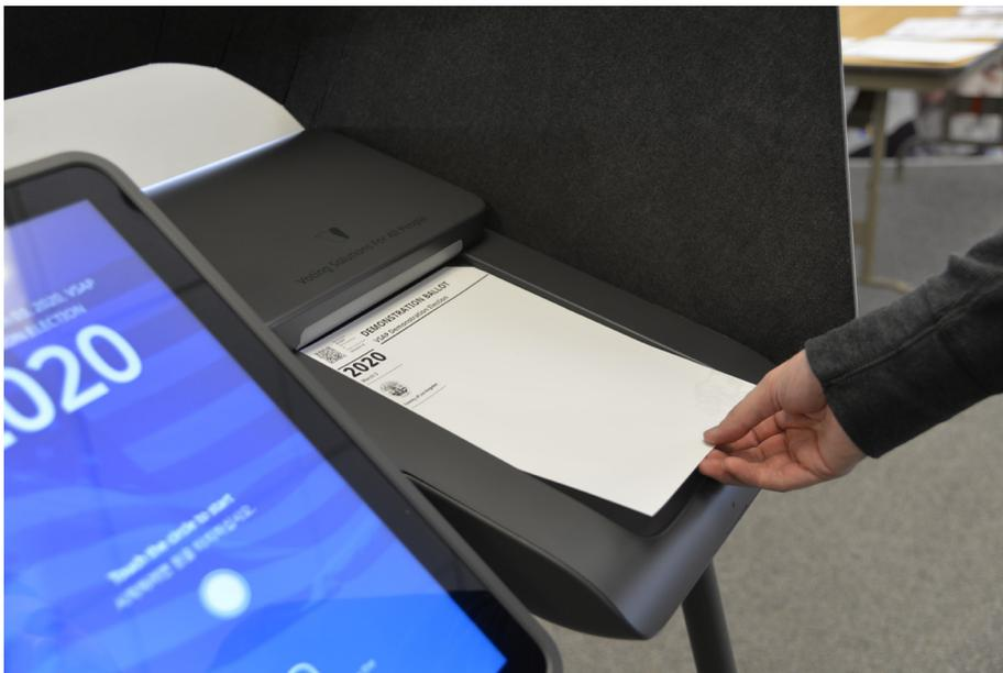
4. If the BMD displays **Paper Jam**, but no paper is in the Scanner (voter may still have Ballot in hand, or it is still sitting in the paper path and can be removed), you will NOT have to break the Zip Tie, remove the IBB Security Seal, or perform Chain of Custody. Follow the steps below:
