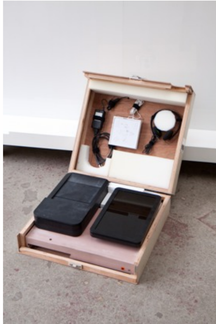
Suitcase contains main electronics unit, headphones, keypad, and power supply.
